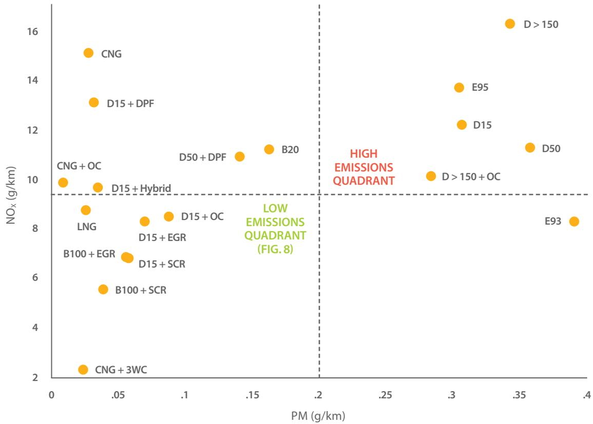
**Figure 8** NO<sub>x</sub> Versus PM Emissions, Close-up on Ranges for Low Emissions Quadrant
