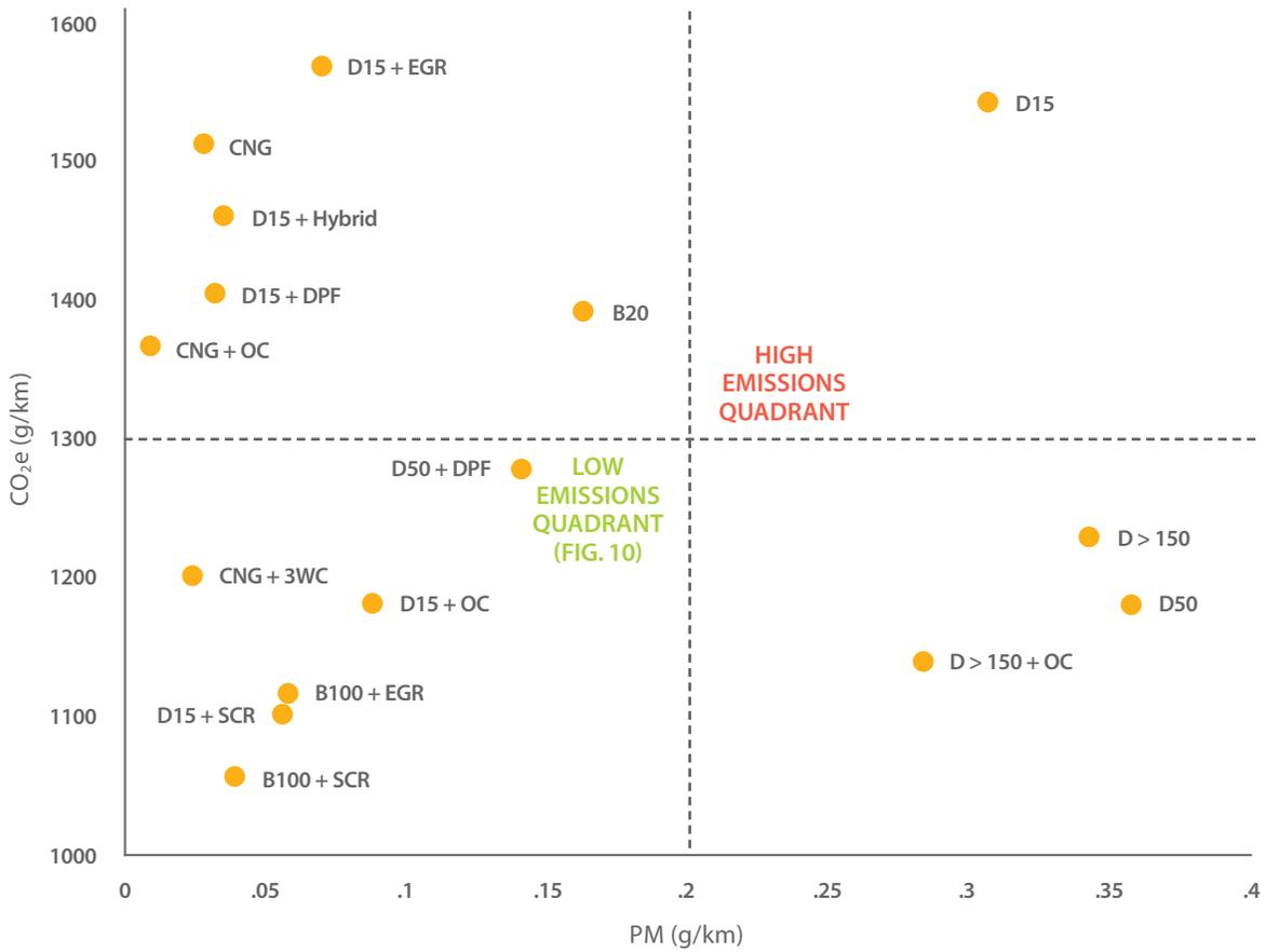
**Figure 10** CO<sub>2</sub>e Versus PM Emissions, Close-up on Ranges for Low Emissions Quadrant
